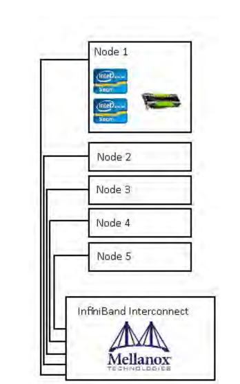
This hardware configuration was chosen to provide a balance between CPUs and GPUs. Xeon processors offer powerful performance across many cores, and Tesla P100 GPUs have incredible parallel floating-point performance. EDR Infiniband offers extremely high bandwidth and low latency for inter-node communication, essential for a modern HPC system. By design, our system runs strictly below the power limit specified by the competition rules, so we will not overshoot the limit during the competition.
